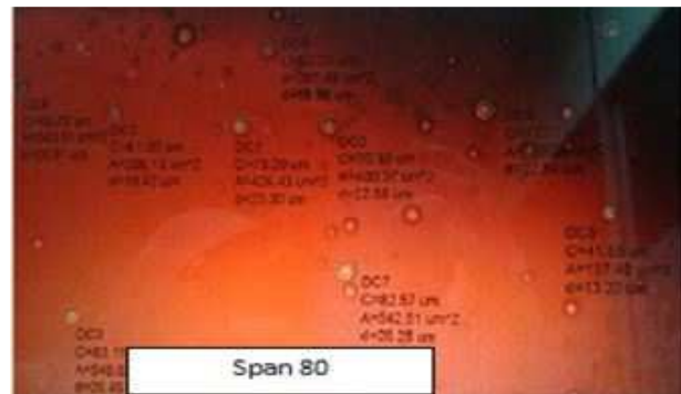
Figure 9: Droplet size with 1.5 wt% Span 80
